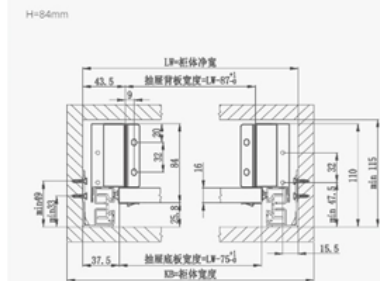
SLIDE RAIL INSTALLATION DIMENSION | 柜体滑轨安装尺寸
